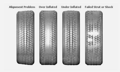
When a tire is underinflated, most of the car's weight is concentrated on the tread that's located just under the sidewalls, rather than being spread out evenly across the full width of the tire. This means that as the tire rolls, the sidewall gets continually flexed
